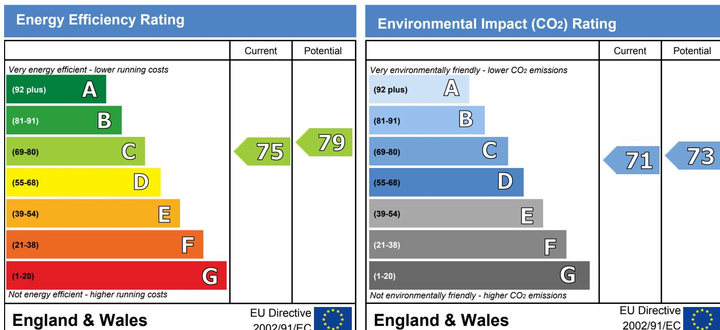
The energy efficiency rating is a measure of the overall efficiency of a home. The higher the rating the more energy efficient the home is and the lower the fuel bills are likely to be.
