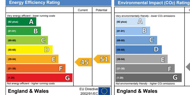
The energy efficiency rating is a measure of the overall efficiency of a home. The higher the rating the more energy efficient the home is and the lower the fuel bills are likely to be.
