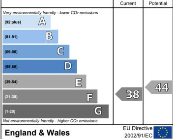
The environmental impact rating is a measure of this home's impact on the environment in terms of Carbon dioxide (CO<sub>2</sub>) emissions. The higher the rating the less impact it has on the environment.
